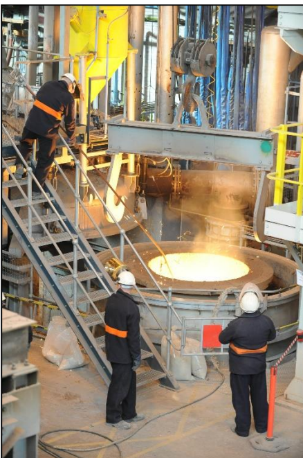
Lifting ladle ready for casting
