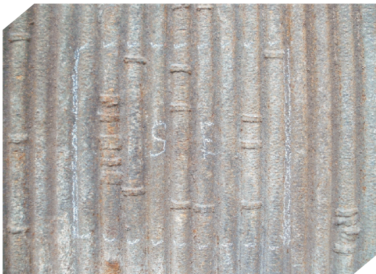
Section of heat exchanger with multiple weld repairs on some tubes
