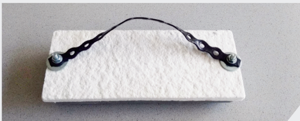
Bare and insulated RFID tags
