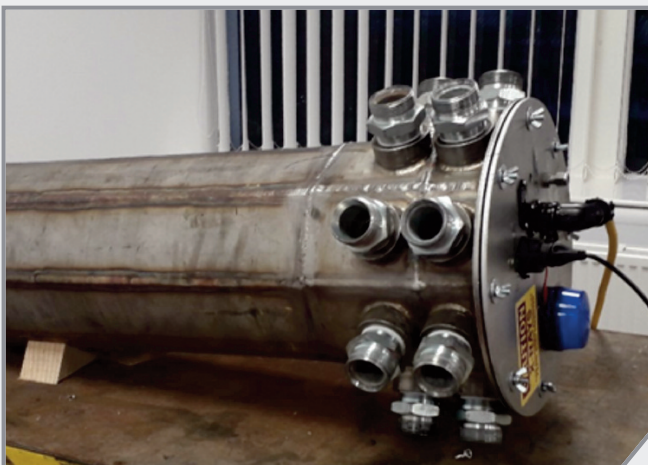
Modified water-cooling housing with XRF internal components installed
