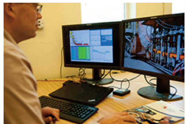
Figure 2. Remote monitoring of caster mimics and data displays whilst watching live CCTV of a cast
