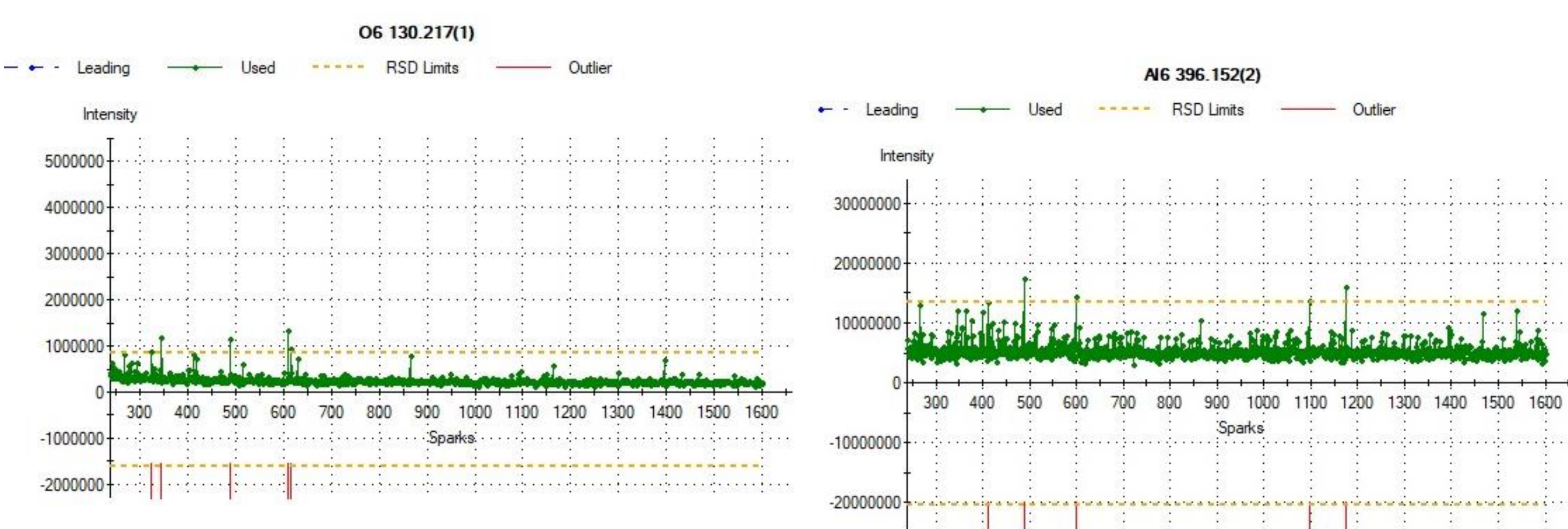
Fig. 1. Single spark evaluation (SSE) of alumina inclusions in steels.
