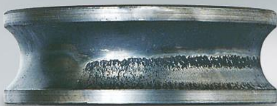
Flaking on bearing inner ring
