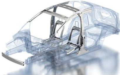
Fig 1 : Automotive body in white Reference : Tata Steel Europe (2005) Automotive - Metallic Coated - Advanced and ultra high-strength steel (Online). Accessed: 01/02/2018
