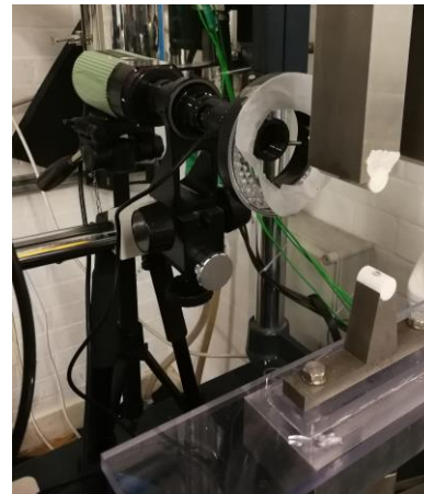
Figure 15. Photo shows CCD camera and inspection tube arrangement.
