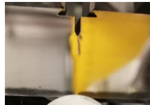
Figure 14. Photo shows notched sample deformed during pre-cracking test.
