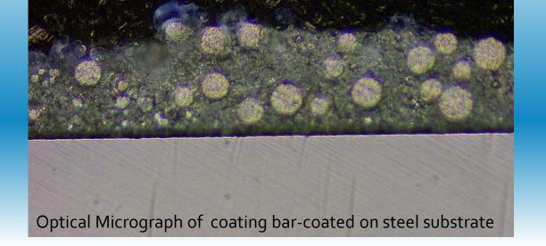
Bar-coating has been used for application. It is found that this gives a more uniform coating. Alternatives for industry will be explored e.g. spraying.
