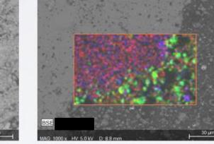
10min20min40minSEM (top) and EDS (bottom) images of coating alloy cured for 10, 20 and 40mins.
