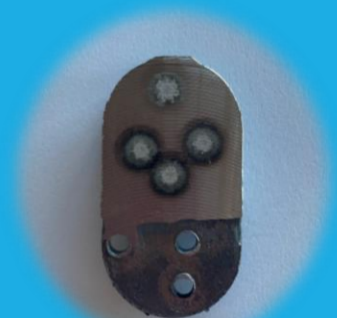
Lollipop sample used in steelmaking
