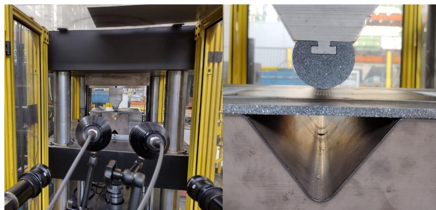
Left: View from DIC equipment. Right: Painted sheet and punch for analysis
