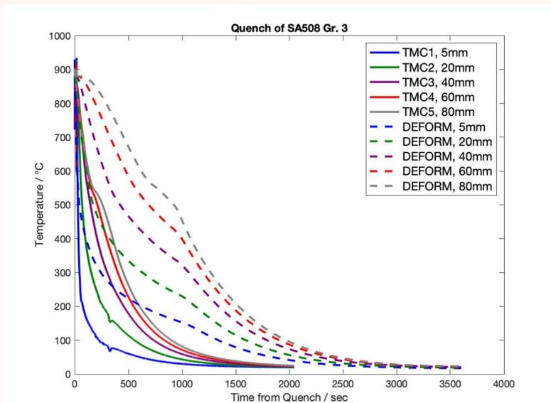
Fig. 3 FEM Modelling of a Jominy End-Quench Test (long profile) plotted against experimental data (short profile). TMC1 – 5 represent thermocouple data.
