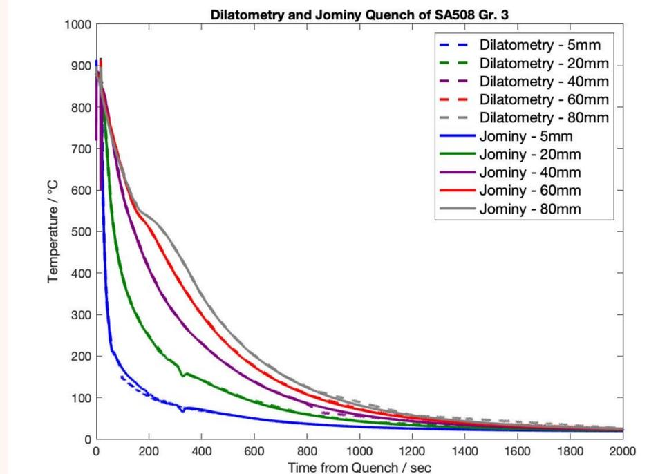
Fig. 4 Jominy End-Quench test data plotted against the profile reconstruction in Dilatometry.
