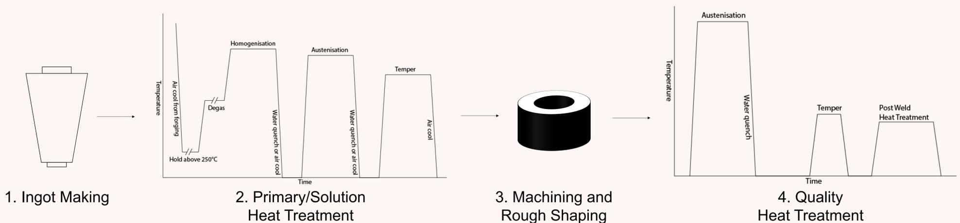
Fig. 1 (Reproduced from [2]) Simplified production route of a typical RPV forging.
