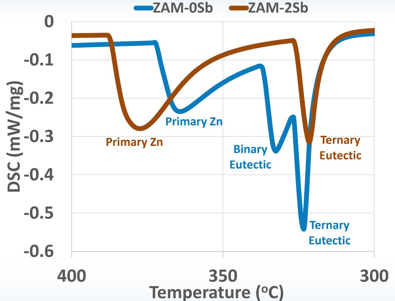
Figure 6 – Differential Scanning Calorimetry (Cooling) Results Comparison for ZAM-0Sb and ZAM-2Sb
