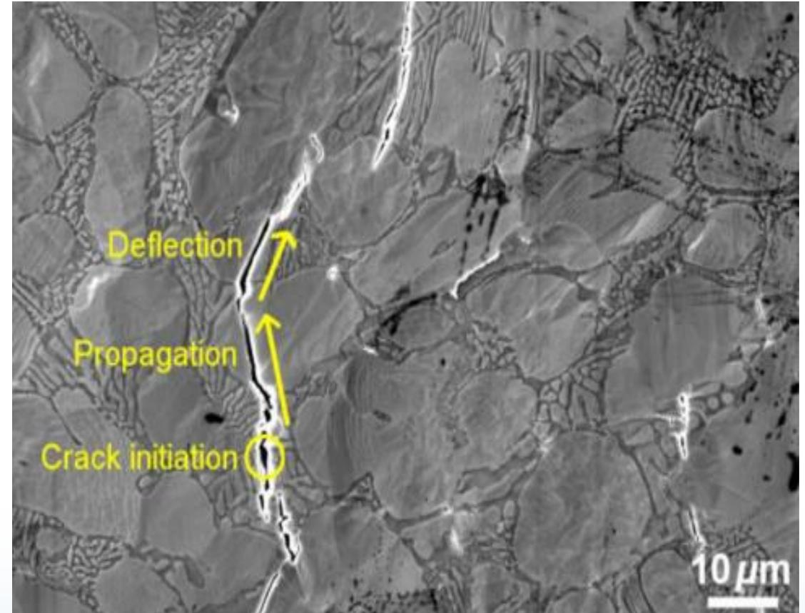
Figure 3 – Cracking in ZAM Coatings [2]
