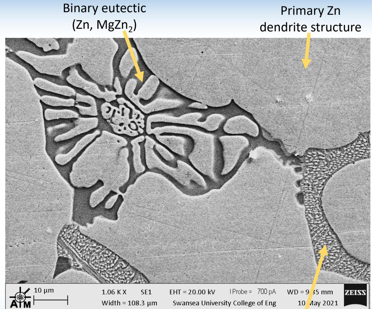
Figure 1 – Microstructure of ZAM Coating
