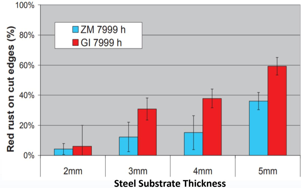
Figure 2 - Appearance of Red Rust on 25 $\mu$ m GI and ZAM Coatings After 7999 Hours in Accelerated SST [1]
