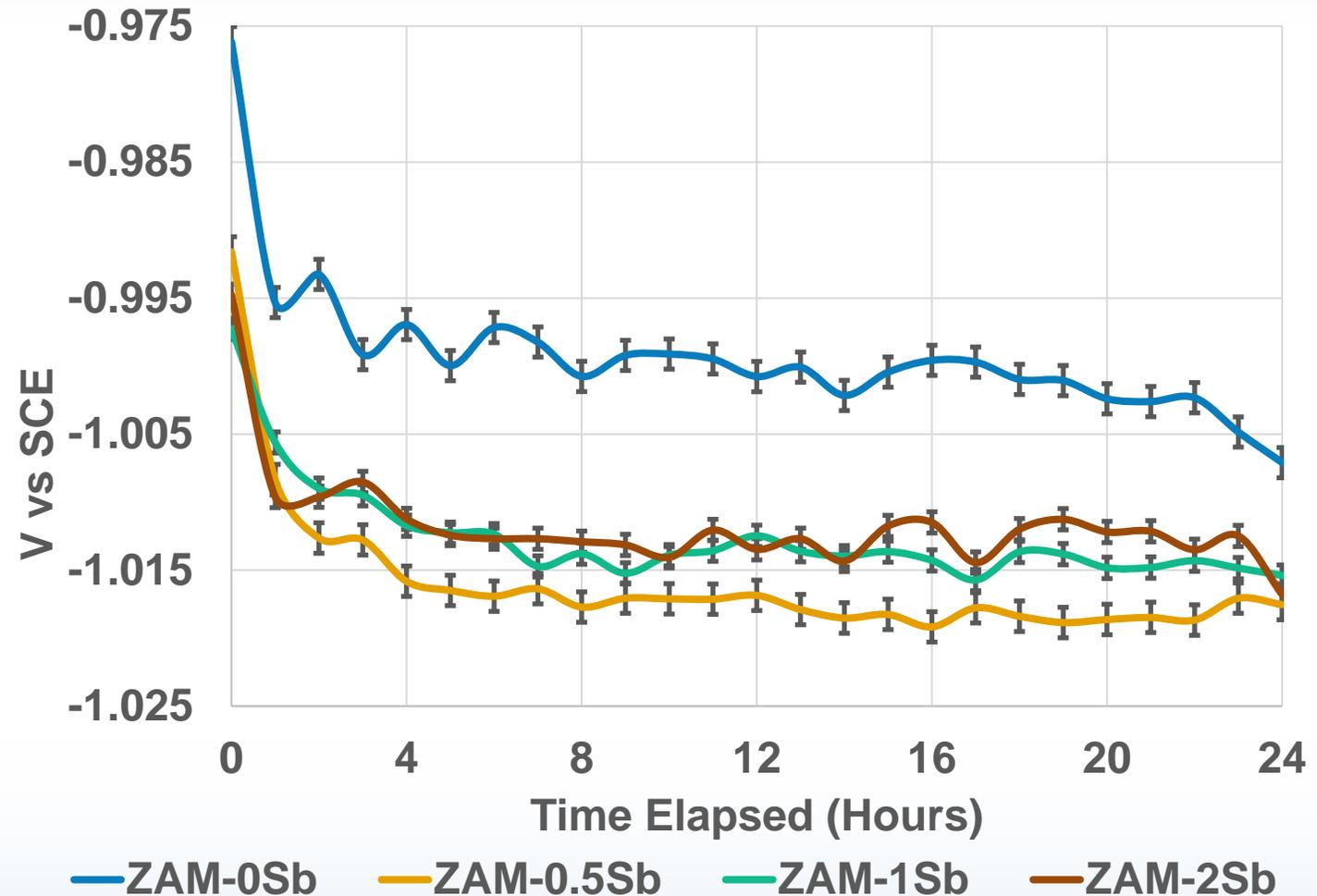
Figure 8 – Open Circuit Potential Results
