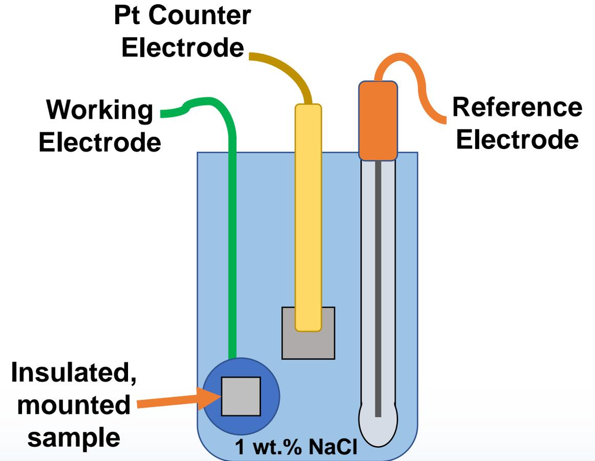
Figure 7 – Corrosion Testing Schematic
