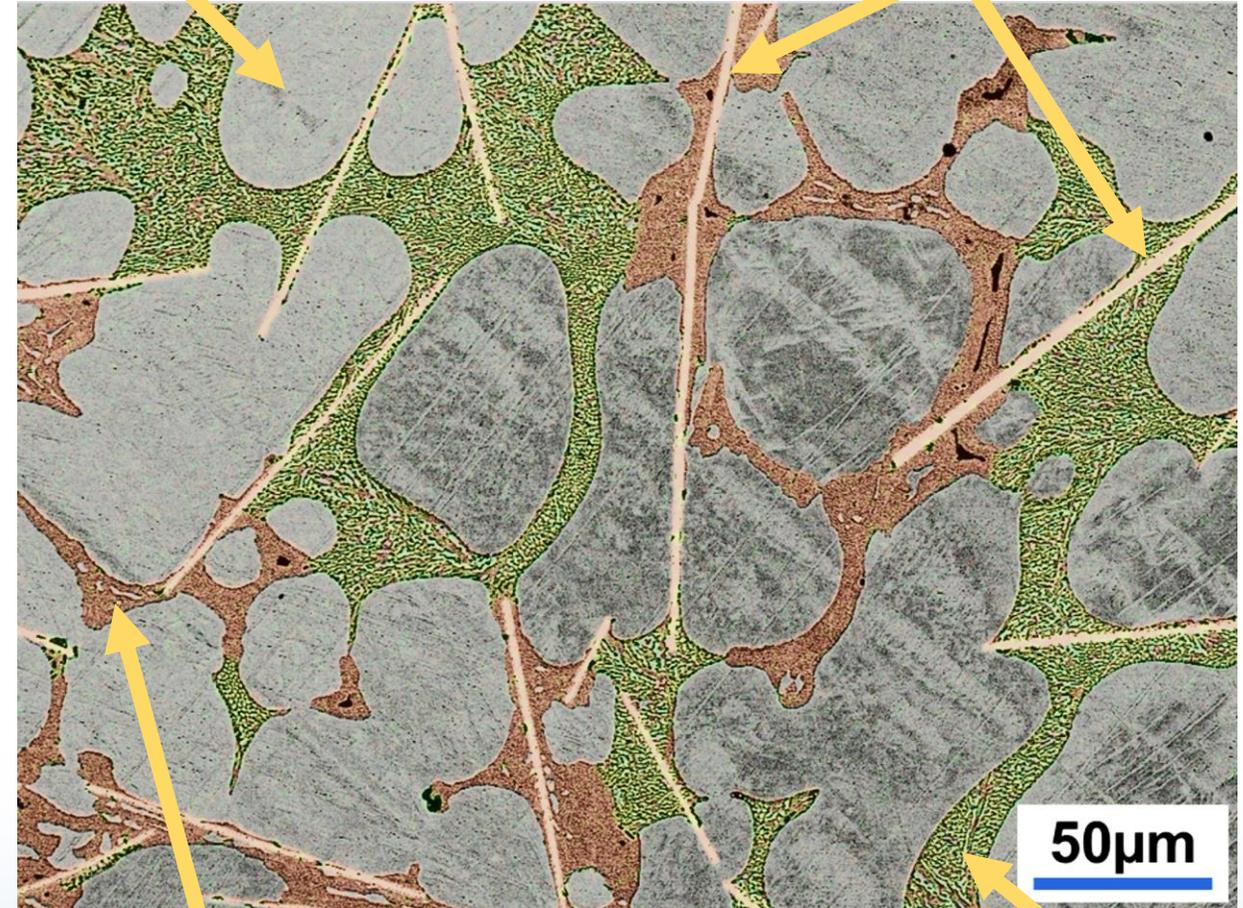
Figure 4 – False colour image of ZAM-1Sb Microstructure
