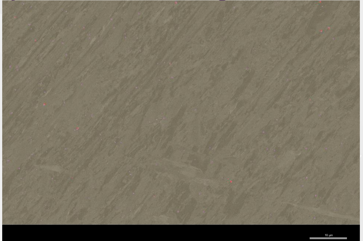
BSE slices of the as-manufactured CPJ7 steel sample after phase segmentation by machine learning
