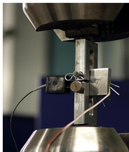
Figure 1: CT test piece assembly on the AMRL Instron 8801 grips
