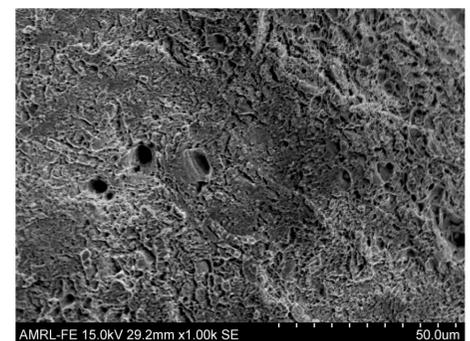
Figure 3: Typical ductile failure with dimple features
