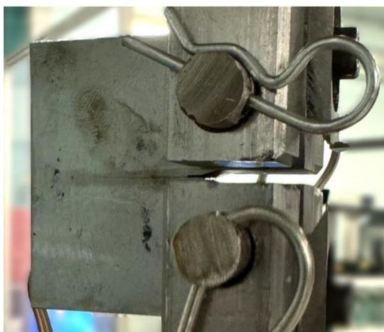
Figure 5: Crack propagating on the CT test piece
