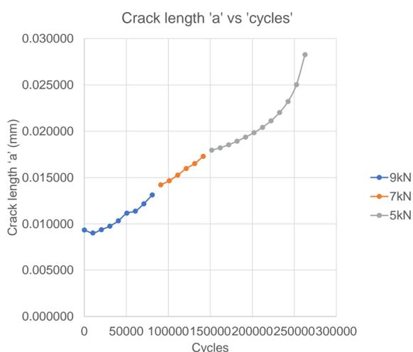
Figure 6: CT test piece crack length a vs number of cycles for three load levels
