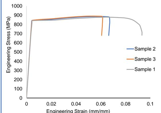
Figure 4: Stress - Strain Curve for S700
