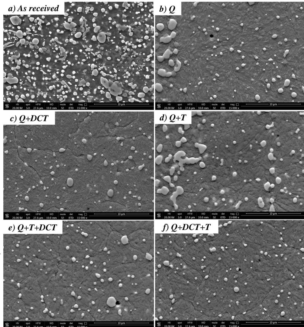
Figure 4: SEM micrographs of the different heat treatment routes (a) As received (b) Q (c) Q+DCT (d) Q+T (e) Q+T+DCT (f) Q+DCT+T
