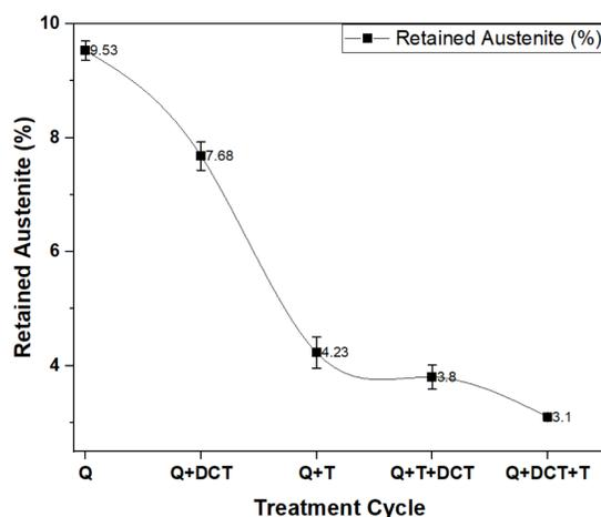
Figure 3: Retained austenite content in the different treatment cycle
