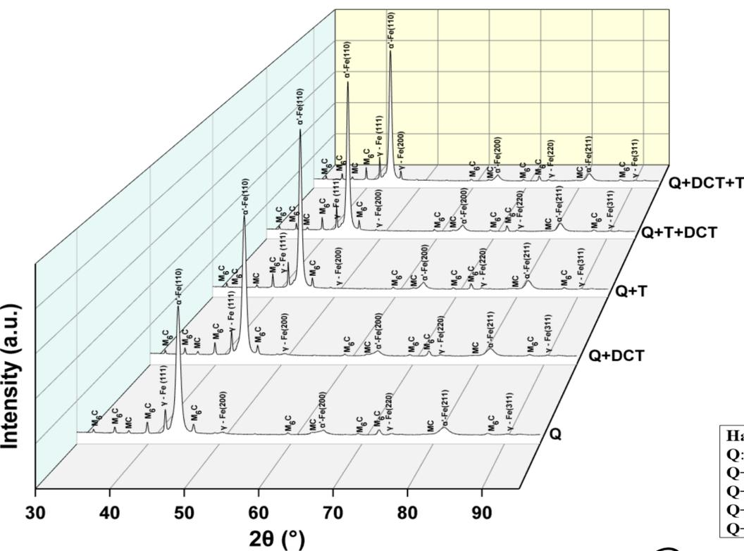
Figure 2: XRD patterns of the different heat treatment cycle
