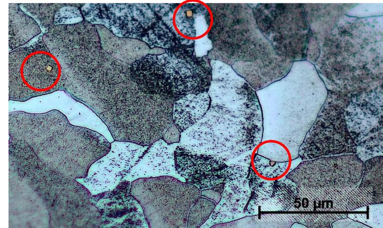
TiNs seen optically on InTRAP carrier material – VIM cast
