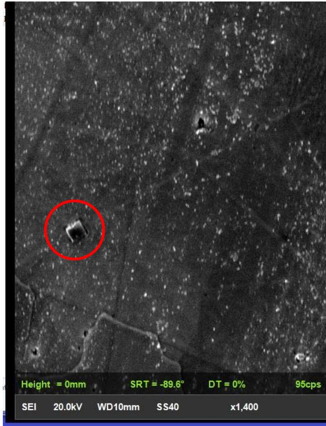
TiNs seen on SEM for 80g route and confirmed using EDS. TiNs formed in 80g route can also be seen optically
