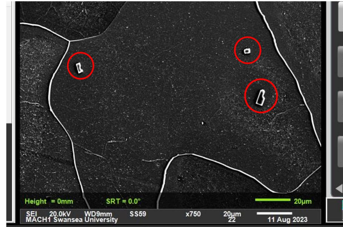
SEM images showing TiN precipitates from high N industrial IF cast, confirmed with EDS
