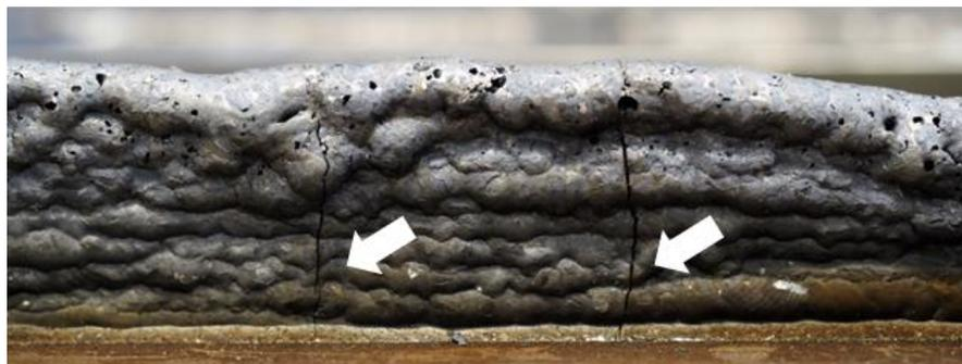
*Occurrence of vertical cracks at multiple locations*
