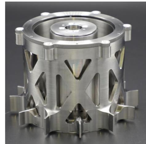
3D printed (LPBF) **Hall Thruster** for spacecraft propulsion
