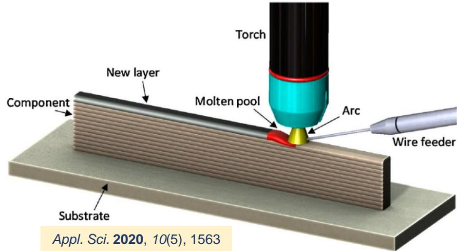
Plasma welding torch with spool wire feeder used
